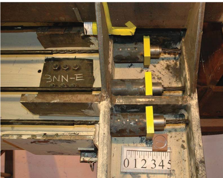
The 4-inch annealed steel tube with wooden disks, or fuse, is designed to be crushed before the post tensioning elements their strength.
